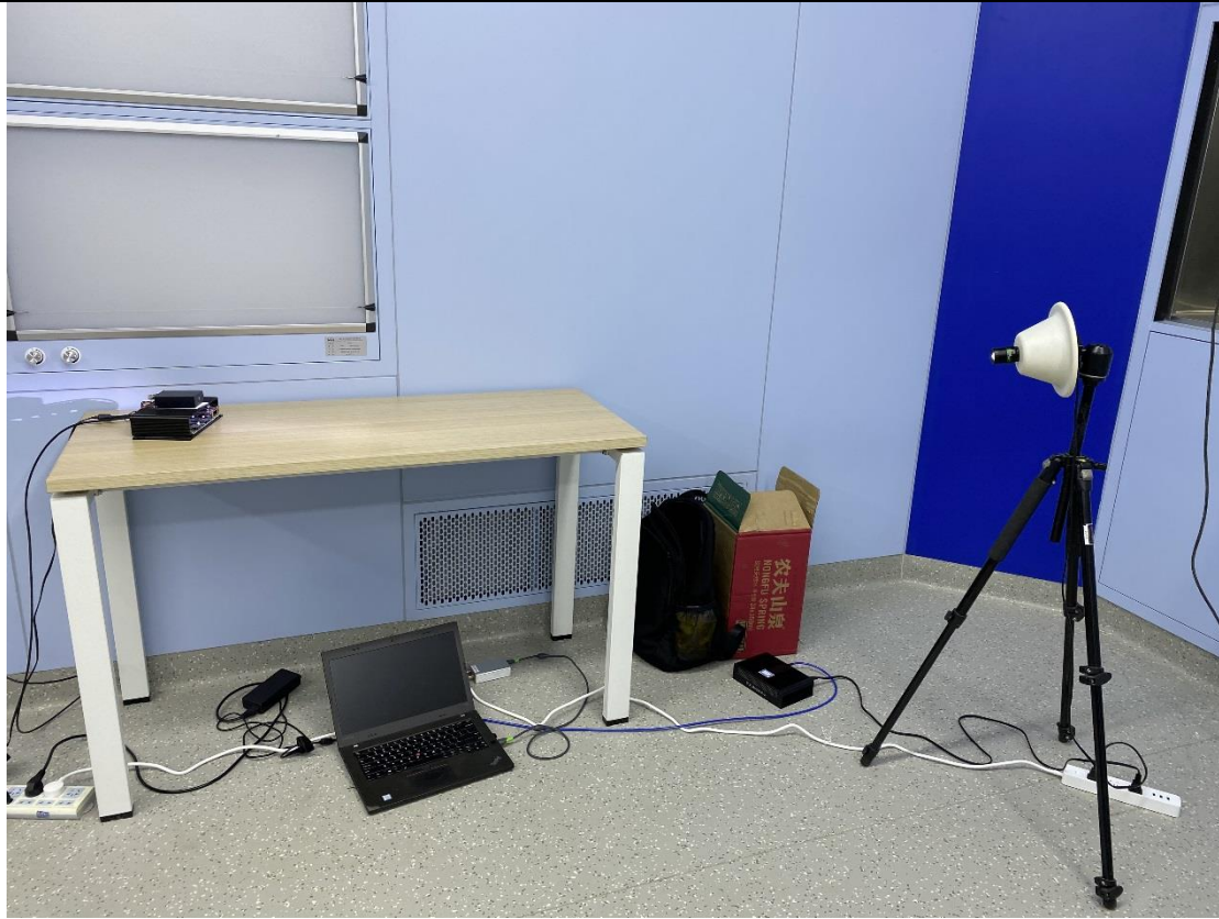
Figure 2: VLC video transmission system used in the digital operation room.
